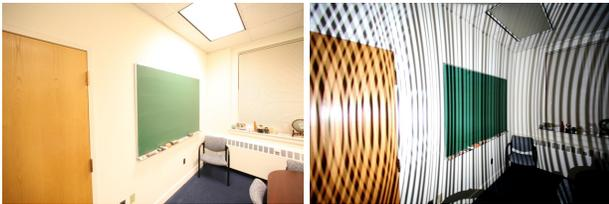
**Figure 3.** Two example images from a scan of an office. Left: an image used to capture the surface color, without the pattern. Right: one of the 15 images acquired with the flashing pattern.
